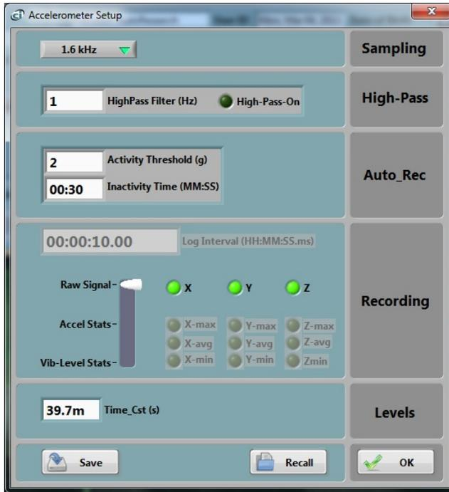
**Figure 8** Typical Setup for measuring Raw Signals
